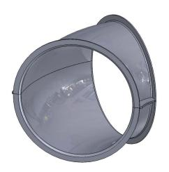
STEP #1- Assemble six elbows. Insert (6) bolts with washers through holes on overlap side of joining flanges. Secure bolts with (6) washers and locknuts on other side of joining flanges then tighten.
