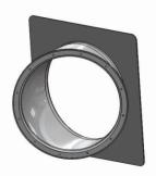
STEP #2- Turn Entry Tube so that it angles to the right side of opening. Center Entry Tube in open-ing and make sure bottom of Entry Tube hole is flush at 5 ft deck level. Secure Entry Tube with (12) lag bolts with washers around outside perimeter of cover plate.
