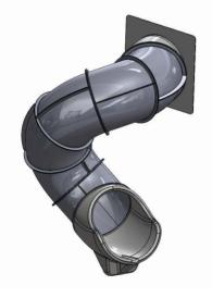
Step #9- Secure over lap end of last 7th Elbow Tube to Tube Slide Exit with (2) 5/16" bolts with washers. Secure two bolts into pressed nuts near the bottom of the Exit making sure the exit is level at both sides. Install 5/16" x 1-1/2" lag bolts with washers through remaining ten holes in elbow flange into plastic of the
