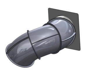
Step #5- Position third elbow with flange end against second elbow overlap end so large joining flanges line up. Turn third elbow counterclockwise one bolt hole and then secure with (12) bolts, (24) washers, and (12) locknuts.
