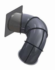
Step # 6- Position fourth Elbow with flange end against third Elbow overlap end so large joining flanges line up. Turn fourth elbow counterclockwise one bolt hole and then secure with (12) bolts, (24) washers, and (12) locknuts.
