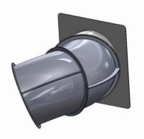
Step #4- Position 3rd Elbow flange end against 2nd Elbow overlap end so large joining flanges line up. Line up ribs of 2nd and 3rd Elbows and then secure with (12) bolts, (24) wash-ers, and (12) locknuts.
