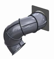
Step # 7- Position fifth Elbow with flange end, against fourth Elbow overlap end so large joining flanges line up. Turn fourth elbow counterclockwise one bolt holes and then secure with (12) bolts, (24) washers, and (12) locknuts.
