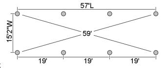
18" in diameter and 24" deep\* for end holes and 16"-18" in diameter and 18" dee p\* for center holes. Positi on 24" sleeves in end holes and 18" sleeves in center holes. If you have I oose/sandy soi I, concrete diameter should be a minimum of 16"-18" for all frames.
